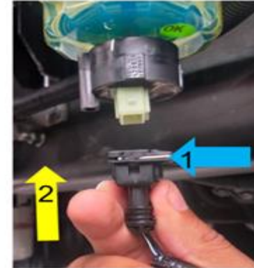
1. Push the connector ring 2. Insert the connector in its seating
