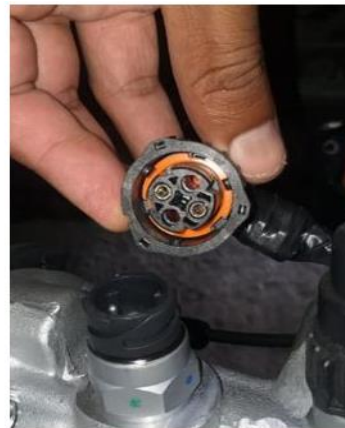
1. To remove, rotate connector lock anti clockwise 2. Pull out the sensor connector
