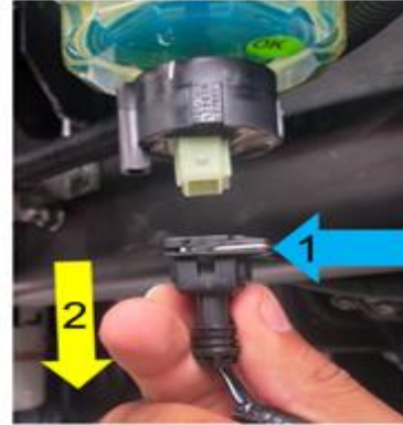
1. Push the connector ring 2. Pull out the connector
